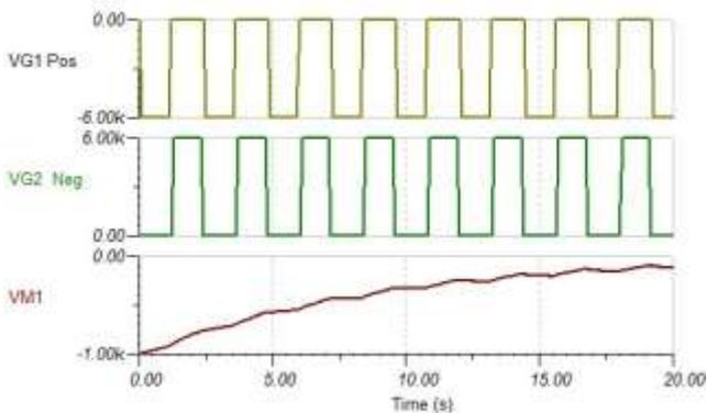
Figure 4 SPICE simulation of a CPM measurement of the Discharge Time of the pulsed DC ionizer shown in Figure 1.
