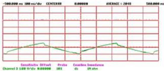
Figure 3. Analog output of the Monroe 288B in the field of a pulsed DC ionizer (Ion Systems 5285e) operating with 1 second ON times.
