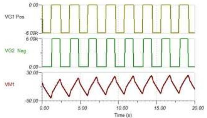
Figure 5. SPICE simulation of a CPM measurement of Balance and Swing setting the initial value on the CPM to 0 V.
