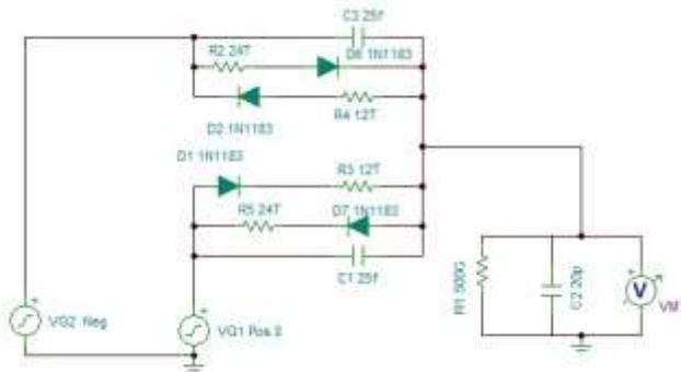
Figure 1. Schematic of simulation model of a pulsed ionizer and CPM system.
