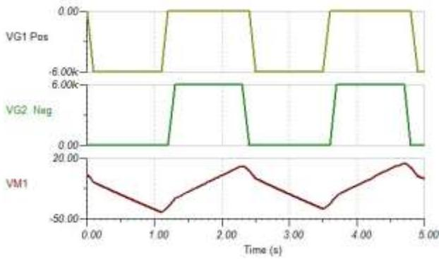
Figure 2. Results of a SPICE simulation of a pulsed DC ionizer. ON times are 1 second and transition times are 200 milliseconds.
