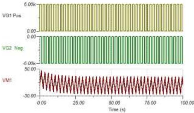
Figure 7. 100 seconds of a SPICE simulation of a CPM measurement of Balance and Swing setting the initial value on the CPM to 0 V. Positive ionizer pulse at the start of the measurement.
