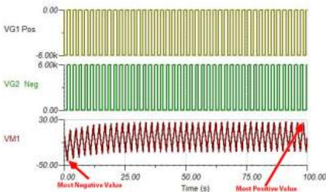
Figure 8. This figure shows what is reported by a CPM following the test procedure in ANSI/ESDA3.1-2006.
