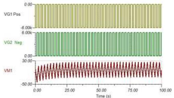
Figure 6. 100 seconds of a SPICE simulation of a CPM measurement of Balance and Swing setting the initial value on the CPM to 0 V. Negative ionizer pulse at the start of the measurement.
